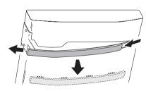
**10.** Unscrew the door handle, turn it 180° and screw it back on to the right-hand side of the door.
